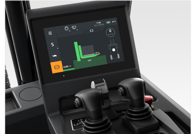
Optional large colour touchscreen display providing vital information and contributing to driver's productivity.
