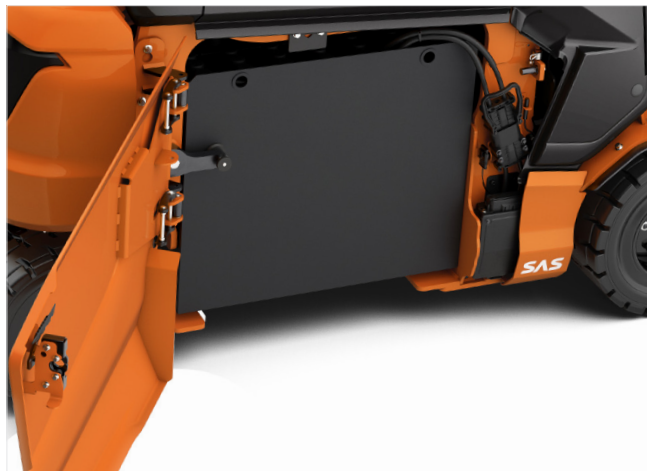
The standard Traigo48 model equipped with lead acid battery has an open chassis design allowing for easy and quick lateral battery exchange/charging.
