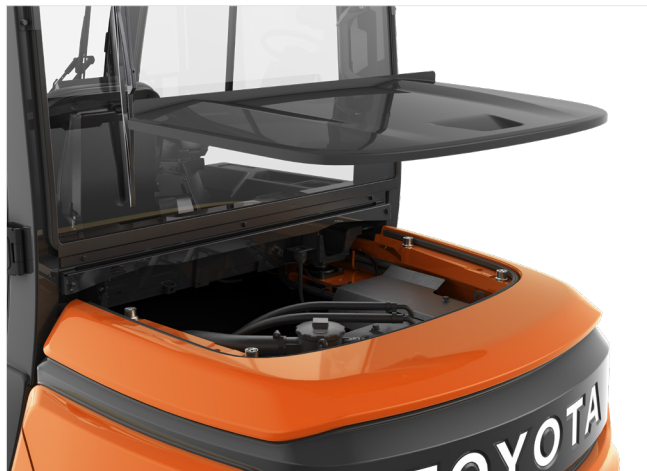
Easy service access via removable counterweight lid, reducing cost and downtime.
