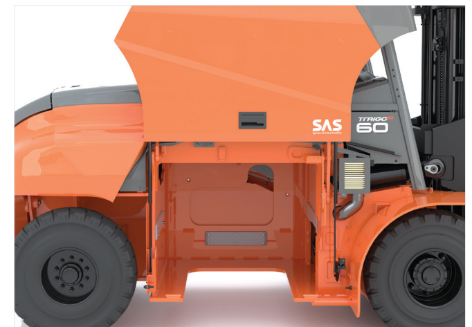
Open chassis design with side panel facilitates lateral battery exchange.
