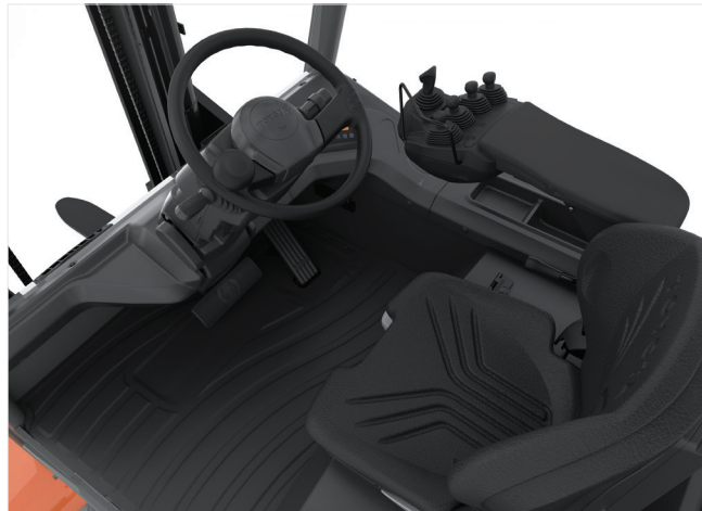
The spacious full floating driver compartment with minimal vibration and low noise offers the driver a comfortable work space.
