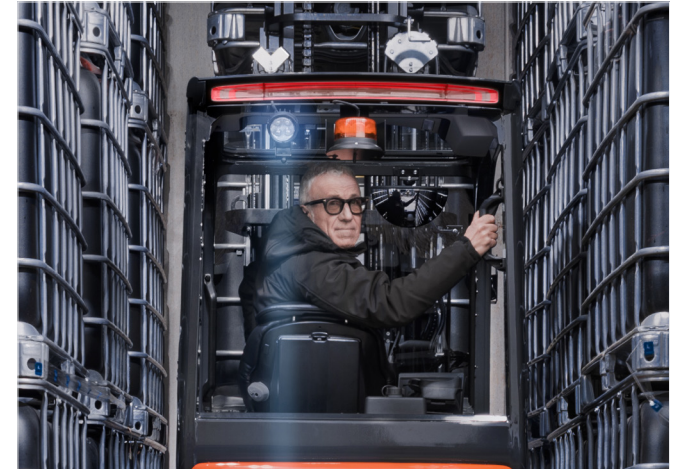
Increasing driver comfort with the rear assist grip when frequent driving backwards (example loading/unloading application) decreases risk of back strain.
