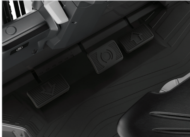
Different pedal layouts are available to fit drivers' preferences. Double accelerator pedals allow the operator to change driving direction with the feet.
